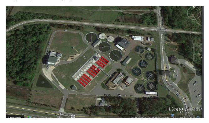
Figure 1 – Aerial View of the CETP with the Activated Sludge Biological Reactors in Red
